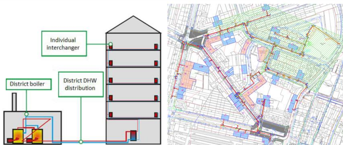
Figure 4: District Heating scheme and network map (source GIR)
