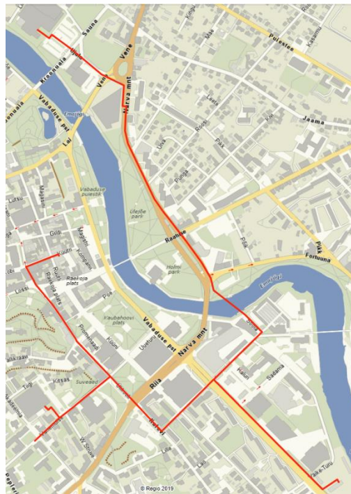
Figure 3: District cooling network in Tartu
