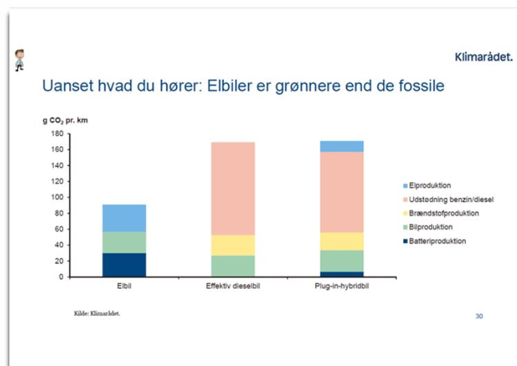
**Figure 3: The electrical vehicle creates only half the carbon emissions per km than a diesel car based on LCA-analysis**
