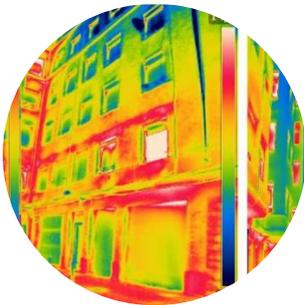
Once retrofitting works have reached their final stage it's time to check if the technical solutions for the façades renovations are performing as expected. One of the best ways to find out is to use thermal imaging technology. The technology has now been used
